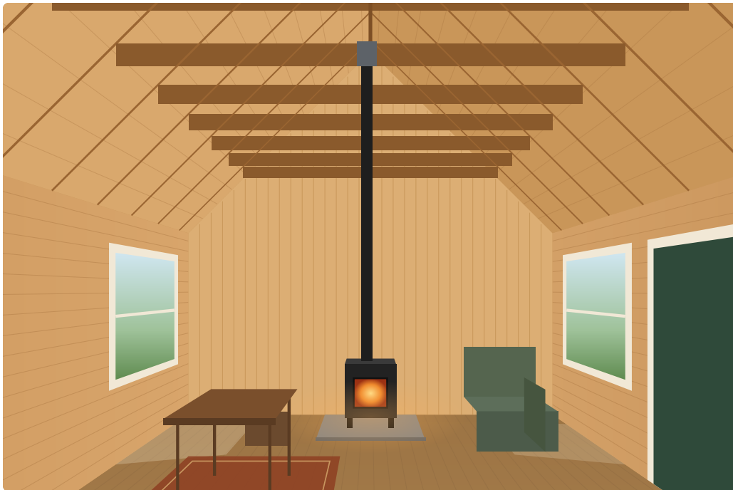
Inside the finished cabin: the open end, with the stove on the center line and a rafter tie on every pair. Illustration.
